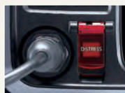
Distress button with a spring-loaded cover
